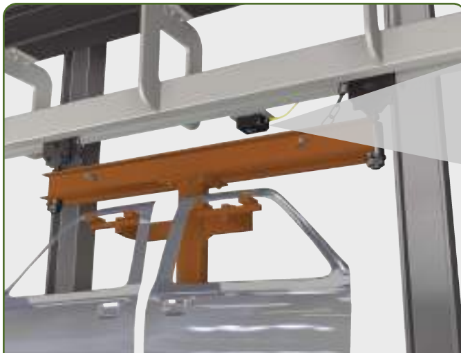
Automotive application – An 871F sensing car door carriers to position them for final assembly.
